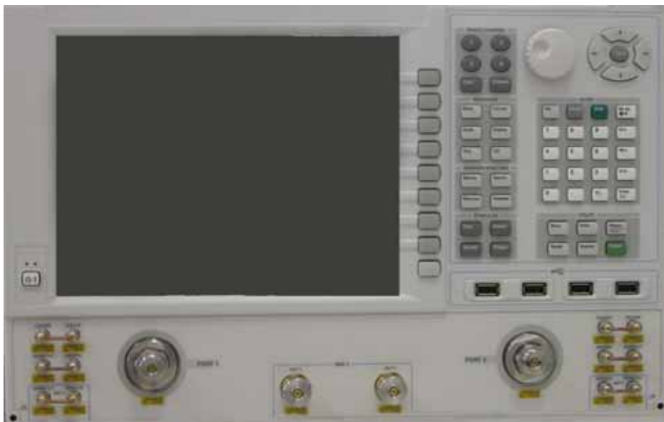
Figure 8 2-Port Front Panel with Internal Second Source
